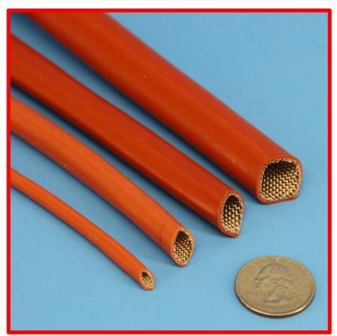
FlameShield™ small diameter firesleeve with Heavy Wall Silicone Rubber coating is designed as a primary insulation sleeve for protecting small diameter wire, cable, lines, hose, and pipe from high temperature, flame and environmental contamination. Recognized by UL / CSA for 240°C, 600V service, and meets VW-1 flammability requirements.
