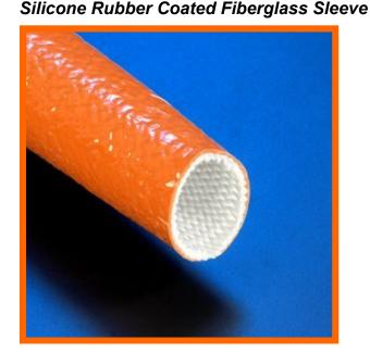
FlameShield™ Marine grade firesleeve allows properly assembled hose assemblies to meet ISO 15540 testing. We also maintain traceability records for customers buying this product. 500°F / 260°C continuous rating and with a 30 minute "Fireproof" 800°F / 426°C rating.
