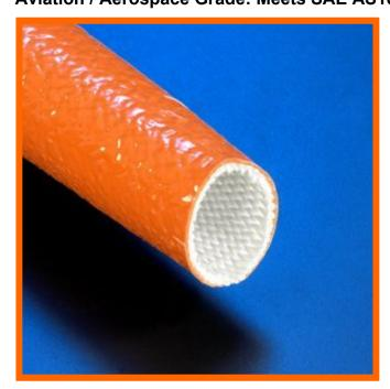
FlameShield™ Aviation / Aerospace grade firesleeve allows properly assembled hose assemblies to meet SAE AS1055D testing. We also maintain traceability records for customers buying this product. 500°F / 260°C continuous rating and with a 15 minute FAA "Fireproof" rating when assembled according to SAE AS1055.
