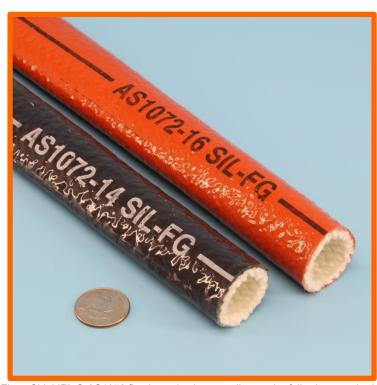
FlameShield™ Aviation / Aerospace grade firesleeve is manufactured to the SAE AS1072 specification. CofC and Test Report available with orders. Our company QMS has been reviewed and accepted by major aerospace OEMs. Allows properly assembled hose assemblies to meet SAE AS1055D testing. We also maintain traceability records for customers buying this product. 500°F / 260°C continuous rating and with a 15 minute FAA "Fireproof" rating when assembled according to SAE AS1055.
